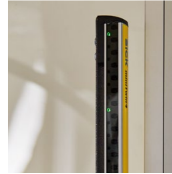
Safety barriers stop the machine immediately if tripped during operation avoiding injury
